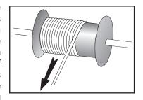
a pipe through the center of the reel and jacking it up until the reel is free from the deck. Rope should never be taken from a reel lying on its side. If the rope is supplied on a coil, it should always be uncoiled from the inside so that the first turn comes off the bottom in a counterclockwise direction.
